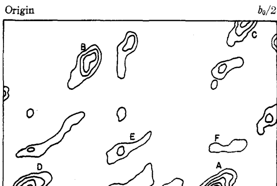
Fig. 1.—Patterson-Harker diagram for the section z = 0 . The peaks represent the following principal interatomic distances: A, Cd-Cd; B, Cd-Cl I , Cd-Cl II ; C, Cd-Cl III (occurring twice); D, Cd-Cl I , Cd-Cl I ; E, Cd-Cl I ; F, Cd-Cl III .
